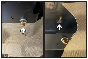
10. Raise hitch into position. Remove lead wires and loosely install a 1/2" whiz flange nut onto each bolt. Do this on both sides of the vehicle.
