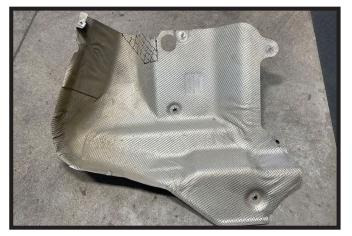
5. Using a reciprocating saw trim the heat shield as indicated to allow for receiver hitch clearance. Repeat this processes with heat shield on other side of the vehicle.
