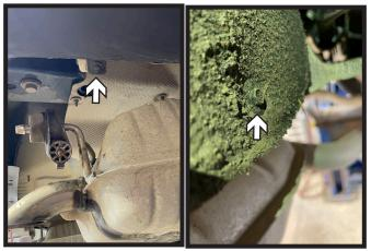
4. Using a 7MM socket, remove the two (2) bolts, one (1) along and one (1) inside the wheel well. Remove heat shield and set aside to be reinstalled later. Do this on both sides of the vehicle.
