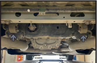
2. Support the exhaust using a jack, stand, or ratchet strap. Using a 10MM socket, remove the two (2) bolts (white) from the exhaust brackets, one (1) on each side of the vehicle. Then remove the two (2) rubber isolators (gray) from the exhaust rods. Lower exhaust to allow for receiver hitch installation.
