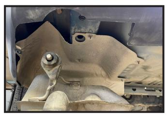
8. Raise heat shield back into place. Do this on both sides of the vehicle.
