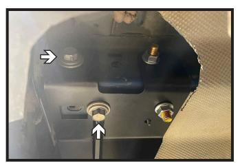
11. Reinstall the two (2) M16 bolts. Do this on both sides of the vehicle. Tighten all bolts
