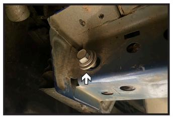
7. Using a 21MM socket, remove the one (1) bolt from the side of the frame. Do this on both sides of the vehicle.
